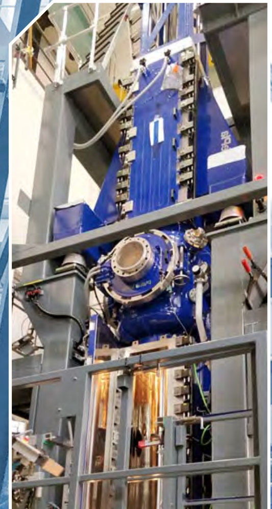
2020 | New float-zone furnace (FZ-30) for silicon crystals up to 8 inches (~ 3 Mio € Invest)
