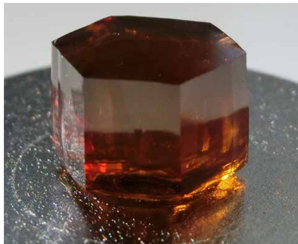
Fig. 2 Sublimation grown AlN crystal (diameter 14 mm) with tungsten aperture.
