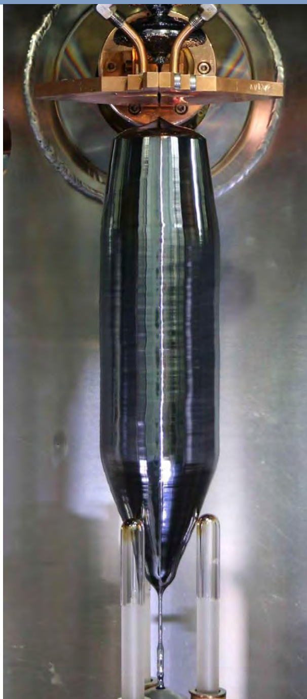
Fig. 1 Dislocation free ^{28}\text{Si} single crystal grown by FZ technique.
