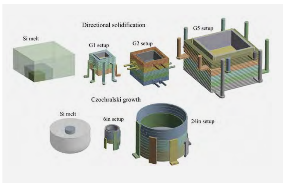
Fig. 4 Crucial parts of DS-Si and Cz-Si crystal growth furnaces equipped with KRISTMAG® heater magnet modules at various scales.
