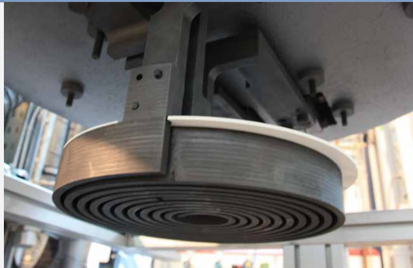
Fig. 3 Image of the newly developed spiral shaped THMM installed at IKZ.
