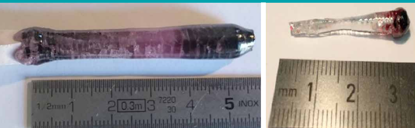
Fig. 2. Left: Result of the first OFZ-growth attempt of Er(14%):Y 2 O 3 performed in a furnace at the company SciDre. The left white part shows the un-melted sintered ceramic feeding rod, the violet part on the right is the as-grown crystal.
