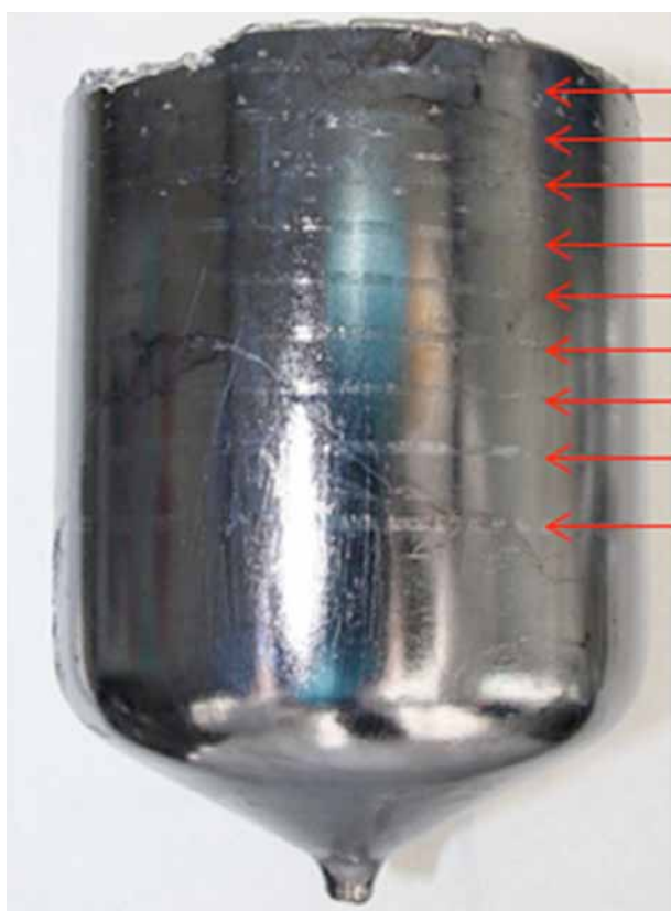
Fig. 2 Image of 4 inch VGF GaAs single crystal crystallized in Top HMM with 9 markers (marked with red arrows).
