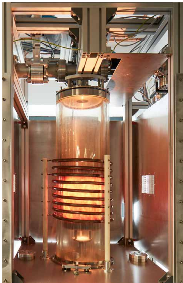
Fig. 1 Image of an AlN growth station built at the IKZ workshop.
