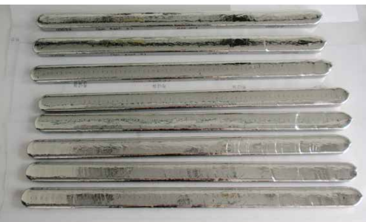
Fig. 1 Zone refined Ge ingots.
