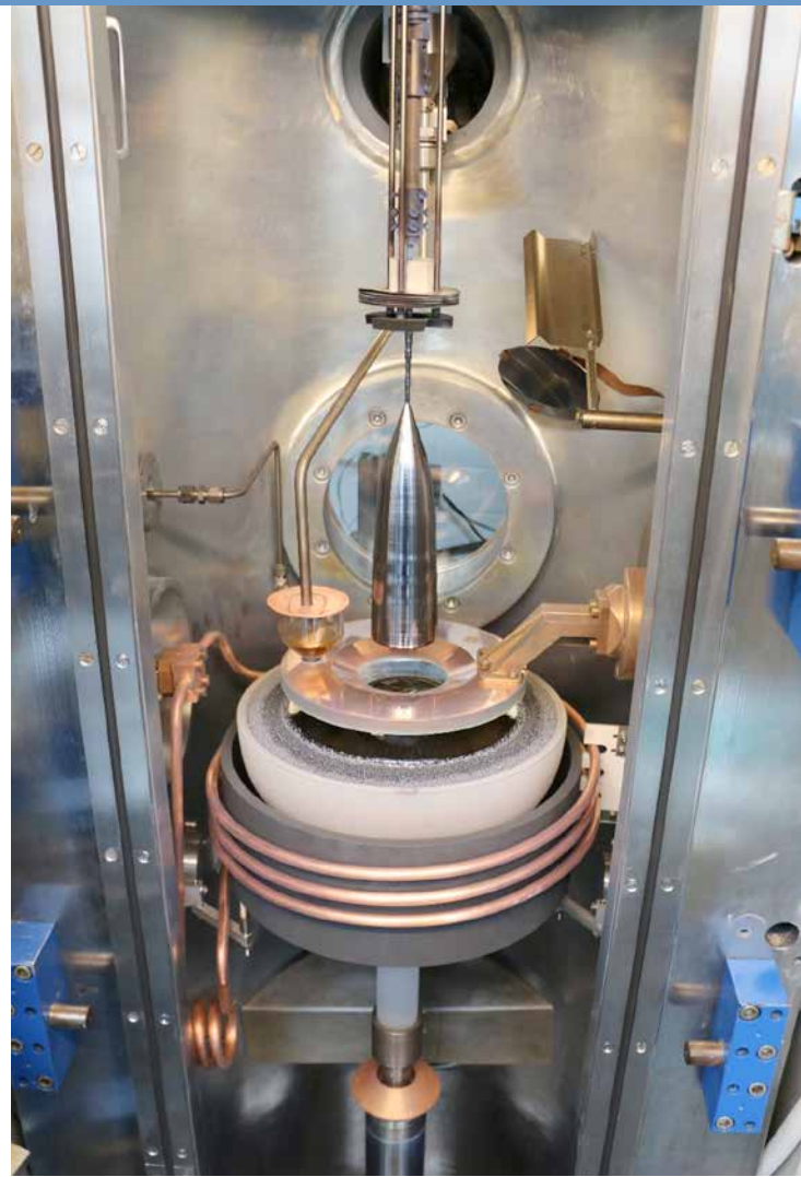
Fig. 4 Si single crystal grown using the developed SiGrEt setup.
