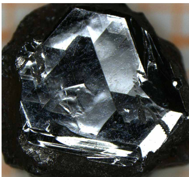
Fig. 2 CuAlO 2 single crystal as nucleated on the solidified melt solution in the Pt crucible
