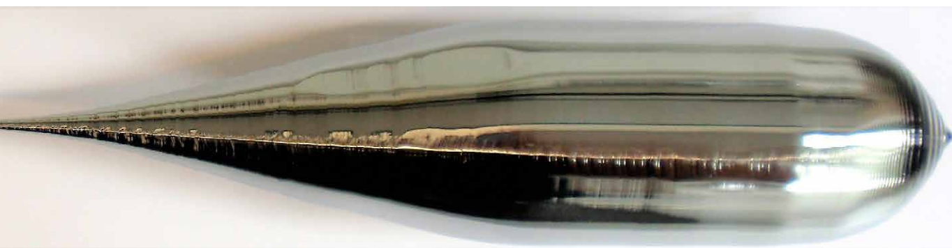
Fig. 1 A 2" HPGe crystal grown by Cz method
