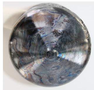
Fig 3 VGF-GaAs crystal with currently the highest total luminosity of 96.2 photons/keV.
