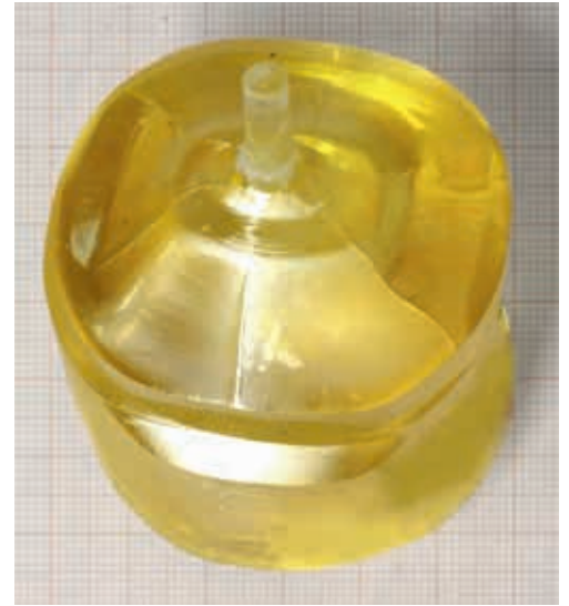
Semi-insulating (Mg-doped, right) and conducting (Si-doped, left) \beta -Ga 2 O 3 single crystals of 2 in. diameter grown by the Czochralski method.
