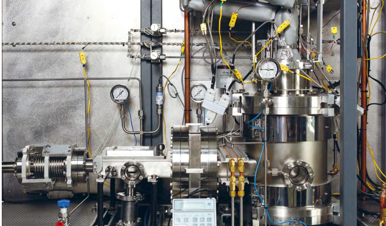
Liquid-delivery spin MOVPE reactor for the epitaxy of ferroelectric (K,Na)NbO 3 thin films Photo: Matthias Kern
