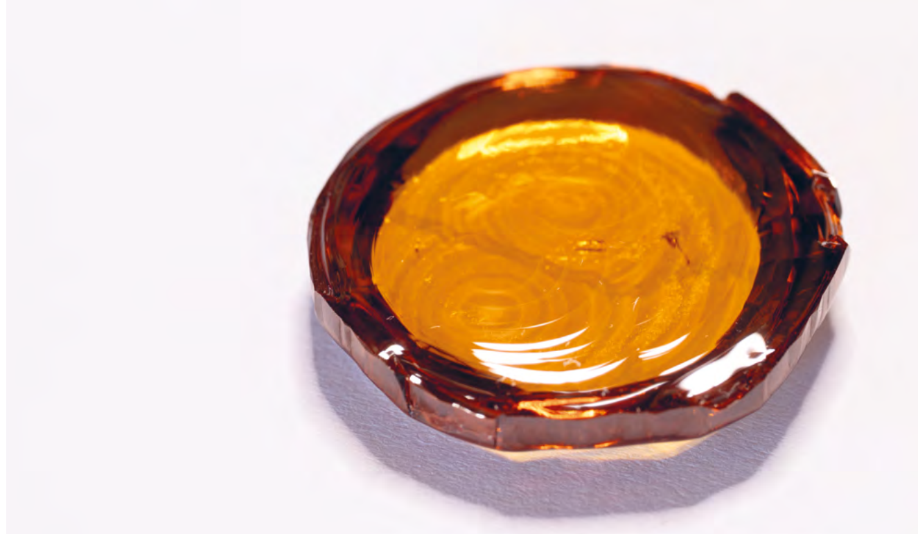
AlN-Crystal with macroscopic growth steps on N-polar surface Photo: HORNNISSEN
