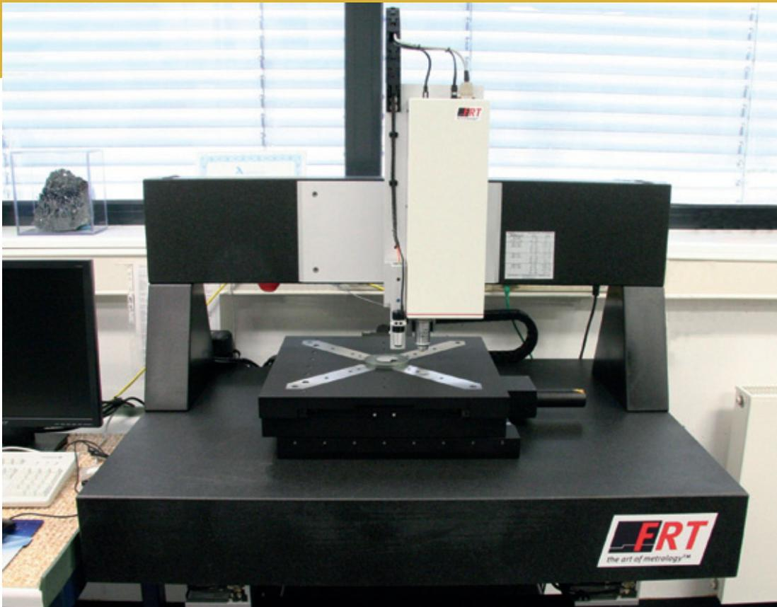
Fig. 1: MicroProf® – Measurement equipment for determination of standard surface parameters (consisting of a chromatic white light sensor and a confocal microscope)
