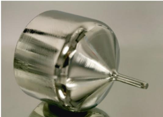
Fig. 1: Germanium crystal grown in a heater-magnet-module
