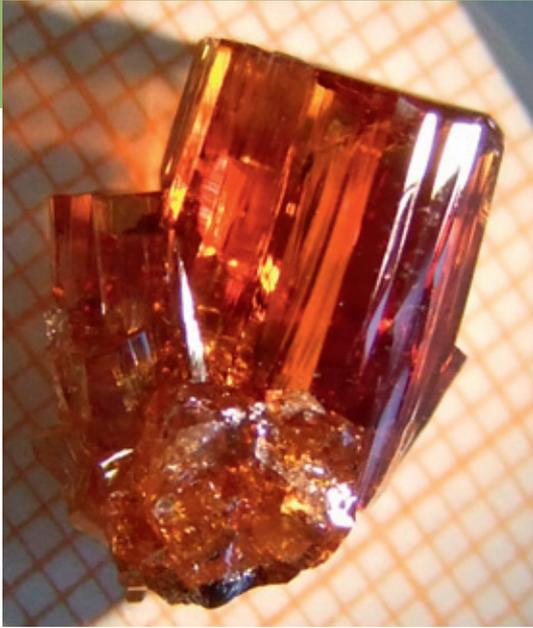
Fig. 2: Isometric AlN crystal grown by seeding on  $\langle 0001 \rangle$ -oriented AlN needles from previous growth runs.
