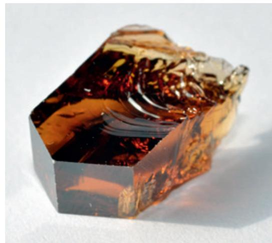
Fig. 3: Freestanding grown AlN crystal (spontaneously nucleated, N-polar c-plane facet shows upwards), size  $13 \times 15 \times 8 \text{ mm}^3$ , HRXRD FWHM about 20 arcsec.
