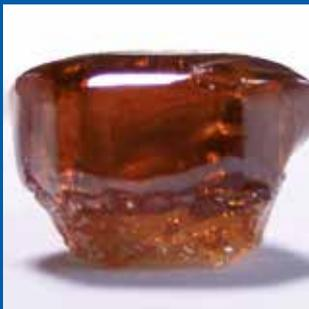
Sublimation Growth of Bulk Aluminium Nitride Single Crystals with High Structural Perfection
