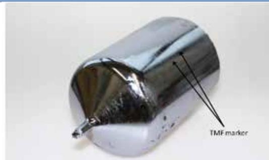
Fig. 3: 4 inch VGF-GaAs single crystal,  $m = 7$  kg,  $\langle 100 \rangle$ -oriented, grown in KRISTMAG®-HMM.
