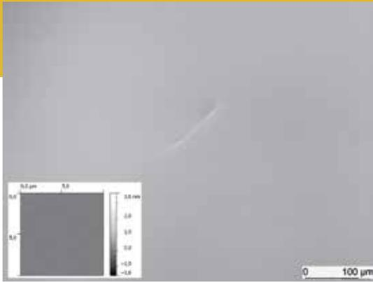
Fig. 1: Micrograph of a chemo-mechanical polished Al polar c-surface of a AlN wafer (insert: AFM image)
