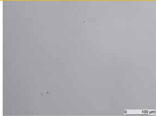
Fig. 2: Micrograph of a defect selective etched Al polar c-surface of a AlN wafer after CMP (etched in KOH melt at 400°C)
