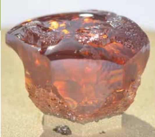
Fig. 4: Homoepitaxial grown AlN crystal ( $\varnothing$  12 mm), final growth interface disturbed by contact with AlN starting material
