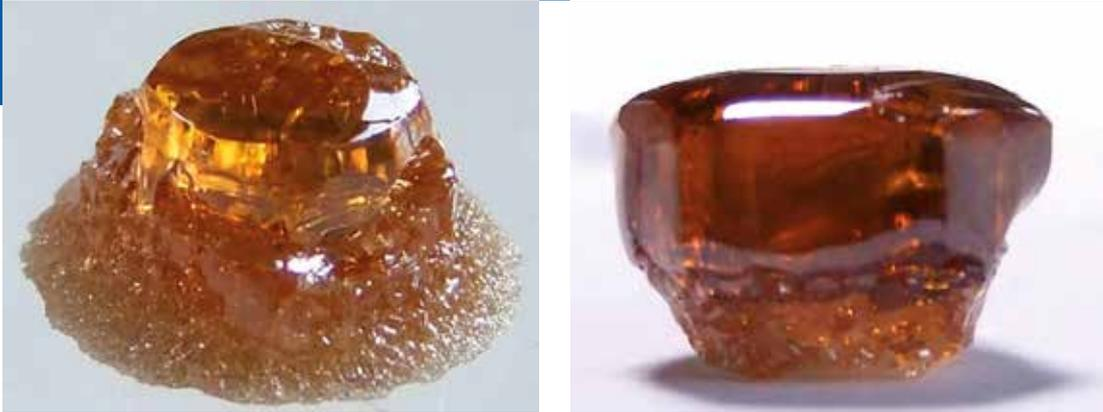
Fig. 7: AlN single crystals grown on N-polar (000-1) AlN wafers,  $T_{\text{Growth}} = 2100\text{ }^{\circ}\text{C}$ , growth time 48 h. Left: crystal with polycrystalline rim,  $\varnothing 6\text{ mm}$ . Right: crystal grown free-standing without parasitic grains using a radiation shield and mesa mounting,  $\varnothing 9\text{ mm}$ .
