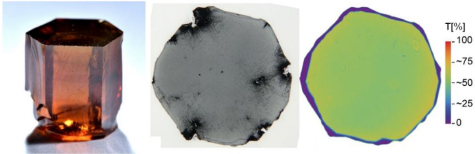
Fig. 1. AlN bulk crystal,  $\varnothing$  10 mm (left). X-ray transmission topograph (middle) and map of optical transmission at 254 nm (right) of a 140  $\mu\text{m}$  thick AlN substrate with  $\varnothing$  10 mm.
