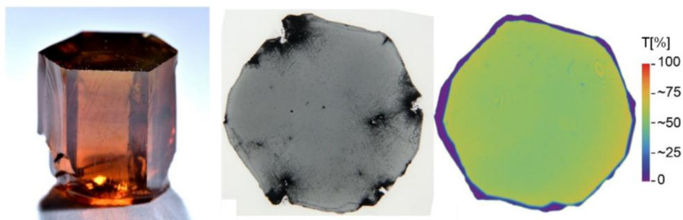
**Figure 1:** AlN bulk crystal,  $\varnothing 10 \text{ mm}$  (left). X-ray transmission topograph (middle) and map of optical transmission at  $254 \text{ nm}$  (right) of a  $140 \mu\text{m}$  thick AlN substrate with  $\varnothing 10 \text{ mm}$ .
