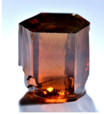
Figure 1. AlN bulk crystal, \varnothing 10 mm. N-polar [000-1] growth direction is upwards.
