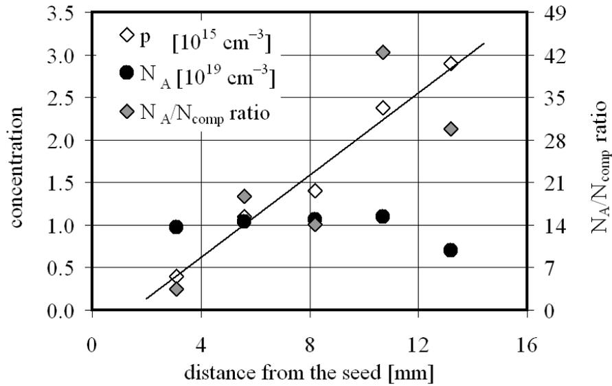
Fig. 1: Axial evolution of the charge carrier concentration  $p$  and the boron concentration  $N_A$  calculated from temperature-dependent Hall effect measurements in a boron doped 6H-SiC crystal. The charge carrier concentration in boron doped SiC samples is linearly correlated to the  $N_A/N_{\text{comp}}$  ratio while the boron incorporation stays virtually constant with growth time.
