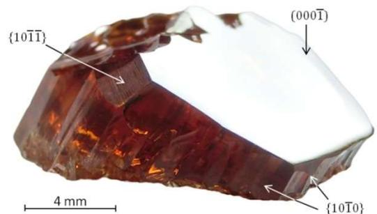
Fig. 4: AlN single crystals grown on (10-1-4) AlN wafer
