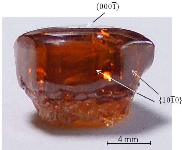
Fig. 1: AlN single crystals grown on N-polar (000-1) AlN wafer
