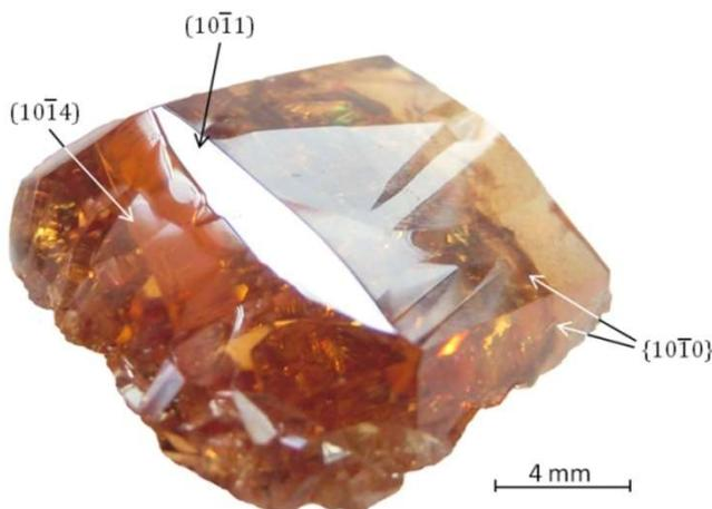
Fig. 3: AlN single crystals grown on (10-1-1) AlN wafer
