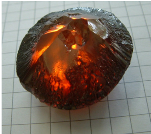
Fig. 1: AlN crystal with rhombohedral facets as well as pyramidal depressions in the center area (on 5 mm grid).
