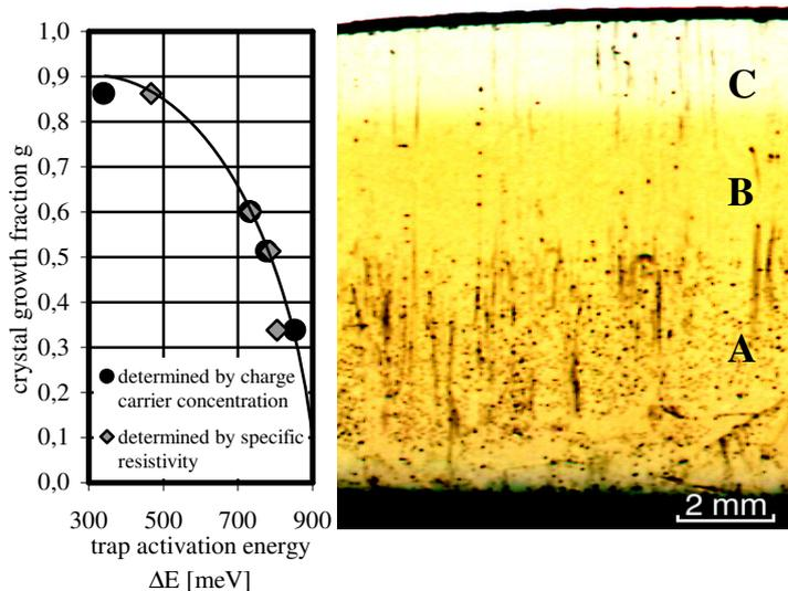
Fig. 1: Cross-sectional cut of a V doped SiC wafer (growth direction is upwards). On the left side, trap activation energies of the respective positions in the crystal are shown. For description of the regions A, B, C see text.
