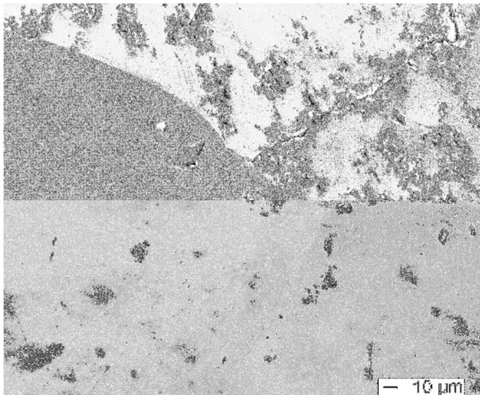
Fig. 1: Wafer surface in scanning electron microscopy. Two neighboring but differently oriented grains demonstrate different density of structural defects (voids and cracks).
