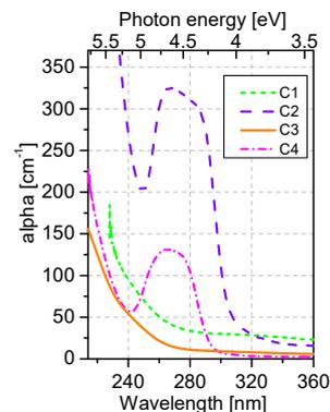
Fig. 2: SIMS values (a) and UV-VIS absorption spectra (b) of AlN crystals grown under different conditions. Crystal C3 reveals  $3[\text{C}] < [\text{O}]$  and  $([\text{C}] + [\text{O}]) < 10^{19} \text{ cm}^{-3}$  which results in  $\alpha_{(265\text{nm})} = 14 \text{ cm}^{-1}$
