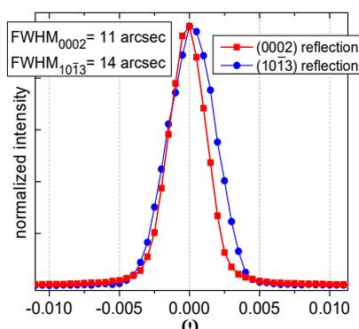
Fig. 1: Rocking curves (open detector) measured with 4-bounce Ge220 monochromator
