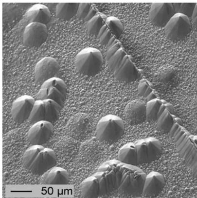
Fig. 2: SEM image of an etched N-polar surface covered by  $\mu\text{m}$ -sized pyramids. Additionally, big pyramids form along cracks and on isolated sites.
