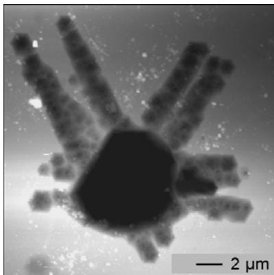
Fig. 1: AFM image of an etched Al-polar surface showing edge dislocation patterns around a bigger etch pit.
