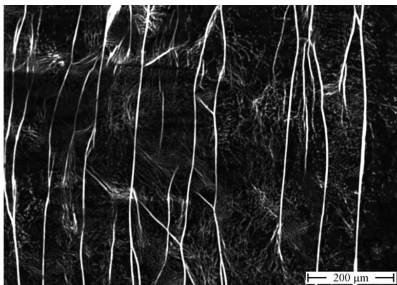
Fig. 1: Panchromatic cathodoluminescence map of a wafer cut perpendicular to the growth direction. Bright lines indicate LAGBs, points indicate single dislocations.
