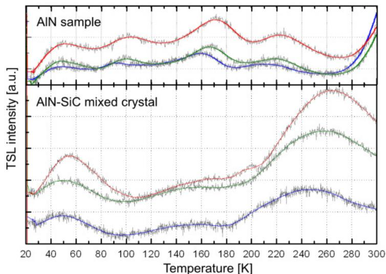
Fig. 1: TSL spectra measured at heating rates of 20 K/min (upper curve), 15 K/min (middle curve) and 10 K/min (lower curve) of a) an AlN sample with silicon and oxygen around  $1 \cdot 10^{18} \text{ cm}^{-3}$  and b) and AlN-SiC mixed crystal.
