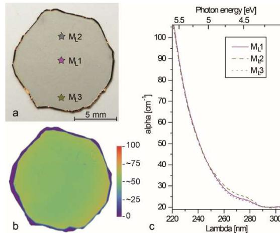
Fig. 2: (a) Optical image of a c-plane AlN wafer (ϕ ~11 mm) with measuring spots; (b) transmittance of this wafer at 254 nm (wafer thickness = 140 μm); (c) absorption spectra at the measuring spots. Except for the outermost rim, the entire AlN wafer shows α<sub>265 nm</sub> = 25-28 cm<sup>-1</sup>
