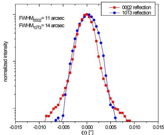
Fig. 3: Rocking curves (semi-logarithmic scale) measured with 4-bounce Ge-220 monochromator and open detector aperture over the full as-grown (000-1) facet area of a typical AlN crystal in the 0002 and 10-13 reflections
