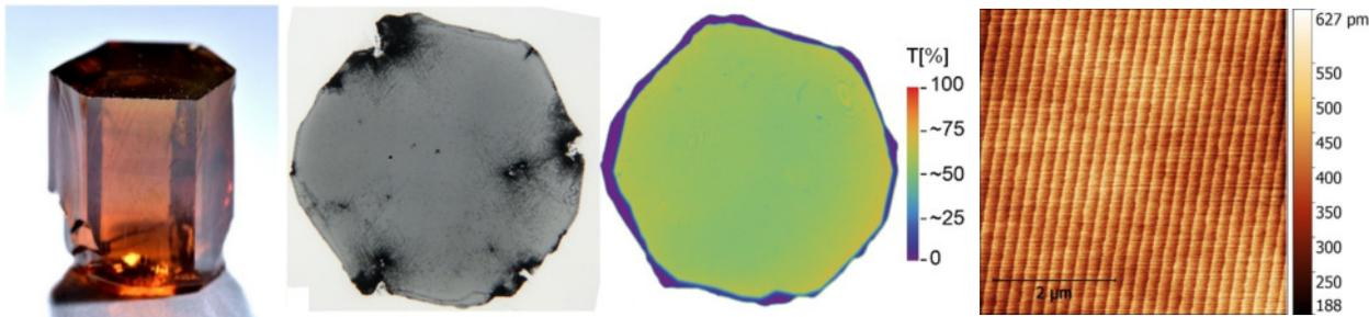
**Fig. 1** AlN bulk crystal,  $\varnothing$  10 mm (left). X-ray transmission topograph (middle) and map of optical transmission at 254 nm (right) of a 140  $\mu\text{m}$  thick AlN substrate with  $\varnothing$  10 mm.
