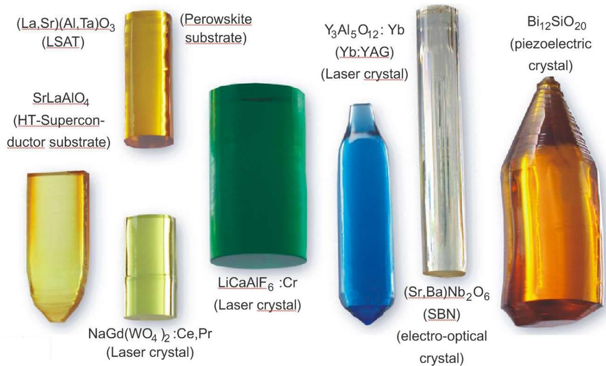
Fig. 1: Oxide and fluoride crystals prepared at the IKZ (selection).
