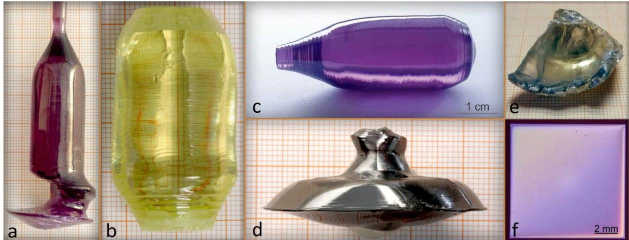
Fig. 1 Selection of some substrate crystals grown at IKZ: (a)  $(\text{Nd,Sr})(\text{Al,Ta})\text{O}_3$ , (b)  $(\text{Mg,Zr}):\text{SrGa}_{12}\text{O}_{19}$ , (c)  $(\text{Nd,La})(\text{Lu,Sc})\text{O}_3$ , (d)  $\text{Tb}_2\text{Ti}_2\text{O}_7$  and (e-f)  $\text{Ba}_2\text{ScNbO}_6$ .
